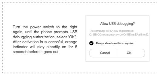
Turn the power switch to the right again, until the phone prompts USB debugging authorization, select "OK". After activation is successful, orange indicator will stay steadily on for 5 seconds before it goes out
